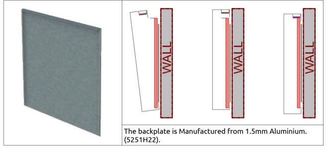
1) Fit backplate to wall. **NOTE:** The **TOP** of the backplate is **15mm down** from the outside top of the frame.
